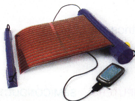
FLEXIBLE VOLTS KONARKA'S FILM, SHOWN CHARGING A PHONE
